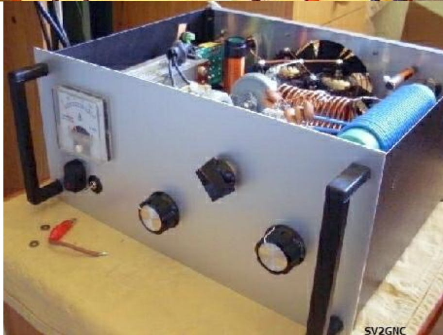
SV2GNC's amplifier, the external anode supply is not shown.
